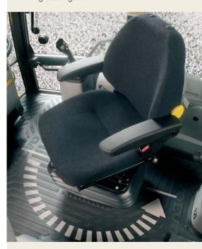
Easily rotate the seat with one hand.
