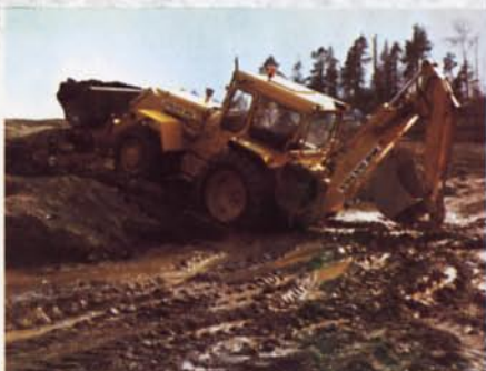
Large clearance angles – good on bumpy terrain
