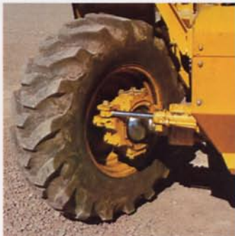
Heavy-duty driven front axle with large wheels
