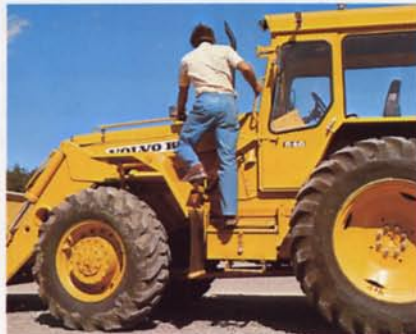
Non-skid footsteps for safe inspection
