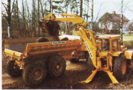
Generous outreach and a favorable carrying angle facilitate loading
