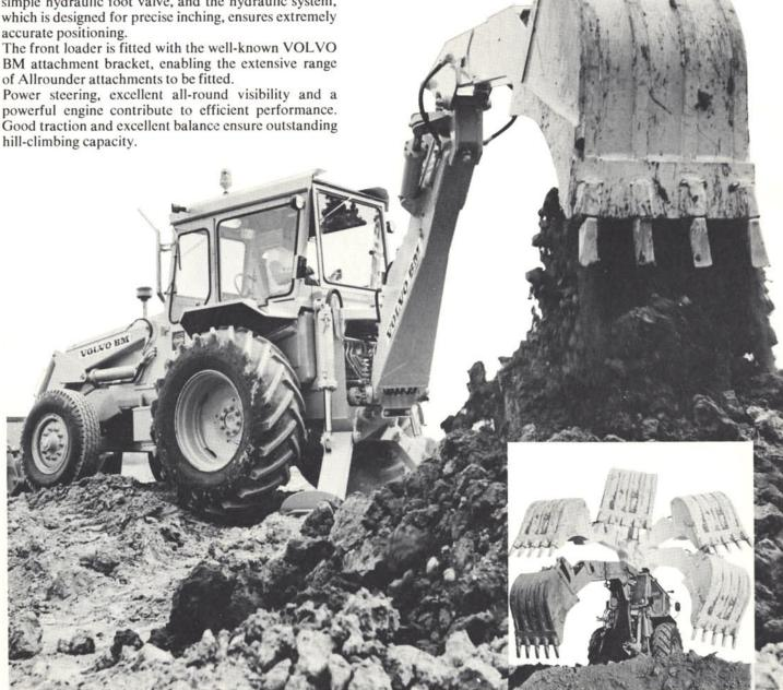
The bucket arm on the VOLVO BM 616 is continuously adjustable on the boom. An infinitely adjustable pedal control enables the arm to be angled laterally at any time during the work cycle.
