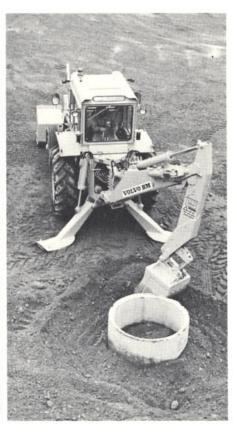
The hydraulically rotatable bucket arm on the VOLVO BM 616 gives the backhoe unit the unique capability of digging and twisting simultaneously. This extra versatility gives greatly improved working efficiency. The VOLVO BM 616 illustrated is digging around an obstruction.
