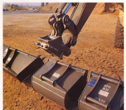
The attachment bracket on the excavator unit comes in two versions, either hydraulically controlled from the cab or mechanically lockable with a key.
