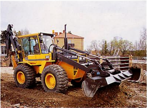
The bucket can be angled a full 114° forward and 51° rearward in the carry position.
