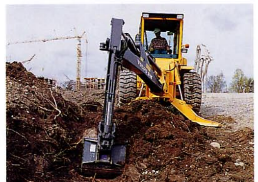
The excavator unit's lateral angulation is completely stepless. You get the best digging angle in all situations.
