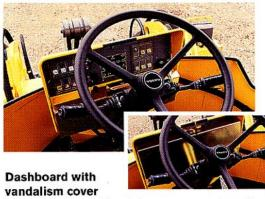
All instruments and switches are grouped on this central dashboard, giving the operator an excellent view of the machine's status. Thanks to their plastic weatherproof covers, the switches are kept dry and clean.
