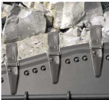
Standard bucket with edge savers
