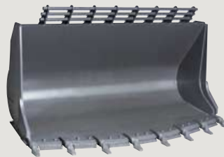
Spade nose rock bucket with teeth
