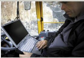
MATRIS stores operational data and shows how the machine is working. This provides valuable information for fault-tracing and service.
