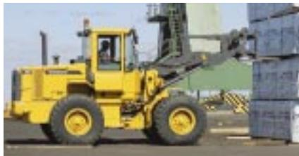
*A small turning radius and exact, load-sensing steering facilitate work in confined spaces.*
