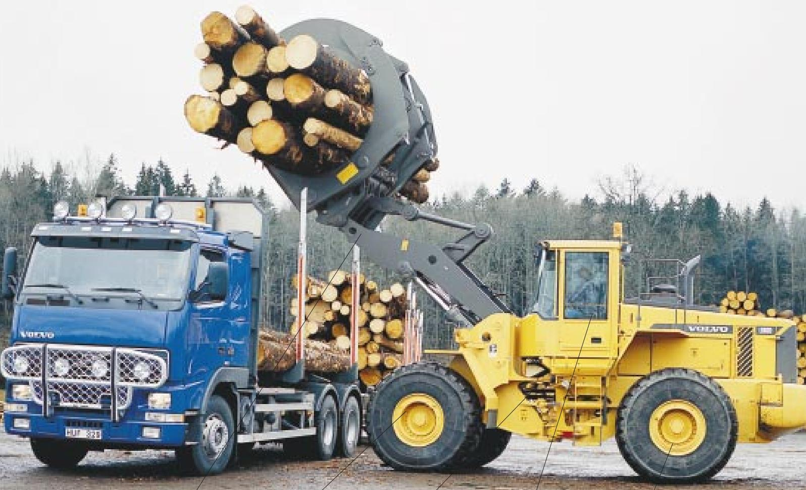
*Volvo's patented TP lift-arm system positions the load's centre of gravity near the front axle. Stability increases and the tipping load is fully utilized.*
