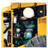
Engine isolated from the cooling system Prevents debris from entering the engine compartment, which reduces the possibility for fires.
