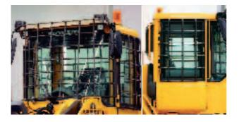
**Window and windshield guards** Protection for both the front, side and rear windows. These guards are custom-made to minimize glass breakage. Radiator grille guard
