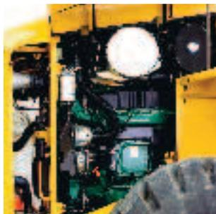
**Engine isolated from the cooling system**
