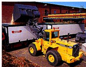
High-dump wood chip bucket.
