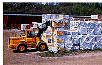
A small turning radius and exact, load-sensing steering facilitate work in confined spaces.
