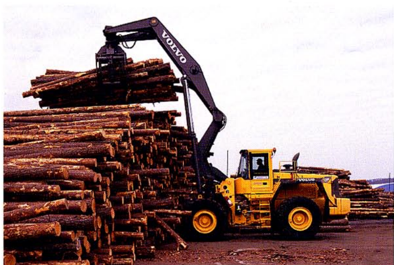
With log pusher and kick-out you can build higher stacks and utilize the storage space on the wood yard more efficiently.
