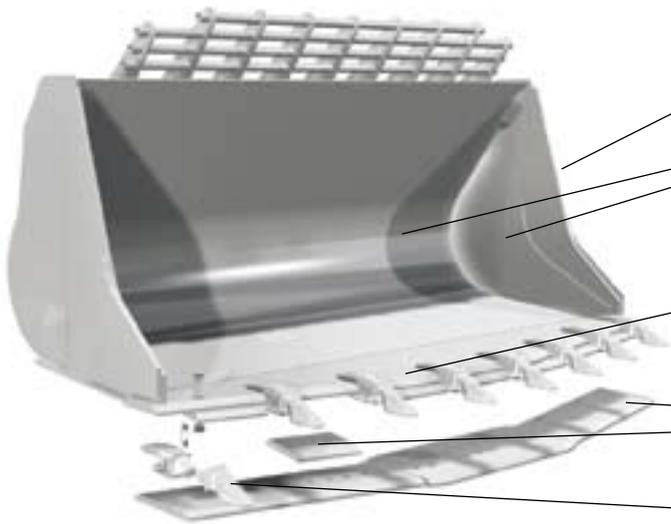
Side cutters with extra hardened and tempered steel wear plates provide high abrasion resistance (up to 500 Brinell)
