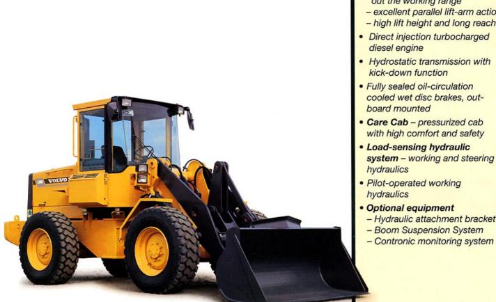
Engine output SAE J1349: Alt. 1 Low emission engine gross 74,5 kW (101 hp) net 71,0 kW (97 hp)
