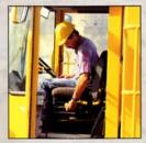
Comfortable operator's seat features adjustable spring suspension, backrest and seat cushion for maximum comfort.
