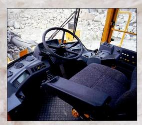
linked to the central warning system, informing the operator immediately of any malfuntion. All information is clearly displayed on the cab console in front of the operator, and faults are indicated by both a flashing warning light and a plain text message.
