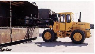
Short work cycles. Good lifting height, long reach and a smooth underside to the loader unit allows wide vehicles to be quickly and easily loaded and unloaded from one side. Parallel lift-arm action and excellent visibility permit safe, sure load control.
