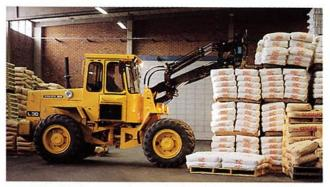
Parallel lift-arm action, articulated steering and a 40° steering angle allows full control of the load and the machine, even when working in small restricted areas.
