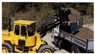
A full bucket every time. High breakout force (54.8 kN) and lifting force (45 kN), plus accelerated rollback provide ample capacity for the toughest jobs and guarantees good bucket filling.
