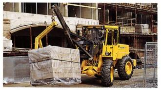
Long reach, good lifting height, ample breakout force and smooth inching action—just what you need for efficient and exacting work with a materials handling arm. In fact, the Volvo BM L30 is in a class of its own when it comes to approved loads when working with this type of attachment.
