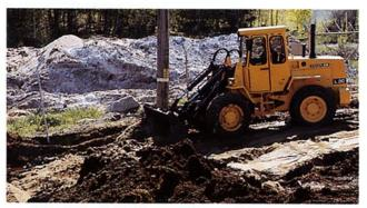
The Volvo BM L30—a productive alternative for levelling small areas. Excellent manoeuvrability, high tractive force and good visibility, together with compact overall dimensions, ensure ideal performance.
