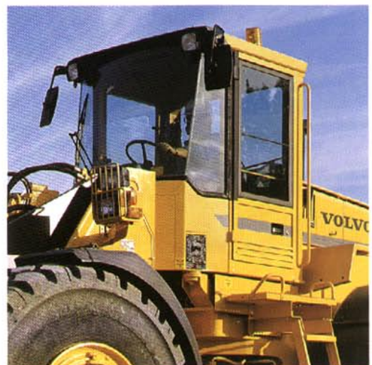
The Volvo BM Care Cab is designed from floor to ceiling to enhance the operator's productivity. The curved windshield without corner pillars and large panes of glass contribute to higher safety on the work site. The Volvo BM Care Cab is, of course, ROPS/FOPS approved.
