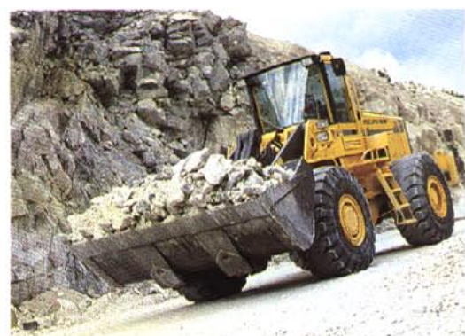
An effective dual-circuit brake system with hydraulic accumulators and fully hydraulic, internal circulation-cooled disc brakes provide excellent braking capacity.
