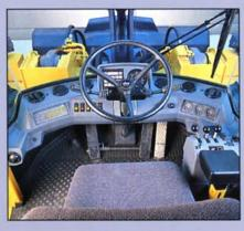
All necessary information can be found on the new instrument panel. Here you also find the Contronic display\*), which provides a continuous read out on the machine's condition. The key operated engine cut-off is of course standard.
