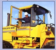
Care Cab. An entirely new cab to meet tomorrow's demands for a good working environment and high productivity. Care Cab is airy and light and comes with large windshields. All interior panels are covered with sound-absorbing materials in coordinated colours.
