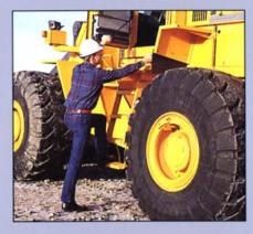
A wide door with a wide opening angle and slip-free ladder with 15 degree tilt makes entering and leaving the cab effortless. Well-positioned handles and footsteps on both sides of the machine facilitate inspection and maintenance.
