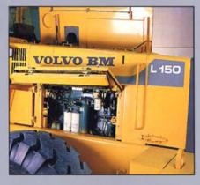
The fuel-injected, 180 kW (245 hp) turbo engine with a maximum torque already at 1200 rpms delivers plenty of power and low fuel consumption. A large radiator and the water-cooled transmission oil makes the machine extra resistant to heat.
