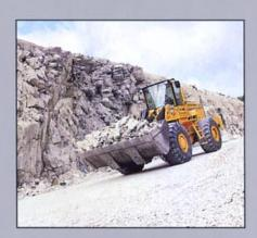
Fully floated axles. The front axle with 100% differential lock, including sealed wet and cooled disc brakes provide a high degree of safety and long life.
