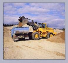
High positioned loader arms with a long reach facilitate loading onto high-sided vehicles. The adjustable, boom and bucket kick out mechanism automatically assumes the proper position for a level bucket and the optimum height for dumping.
