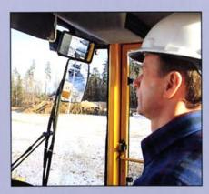
Large, easily adjustable rear-view mirrors ensure good rear visibility. The mirrors are positioned high so as not to block forward visibility. The L150 gives the operator complete control over his surroundings.
