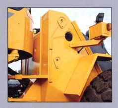
Quick and easy maintenance ensures more reliable operation. That's why all lubrication and control points have been positioned for easy access from the ground. Sealed bearings also help to increase operational safety and longer life.
