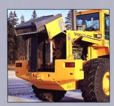
Large, gas strutted hatches for the engine compartment facilitate service and inspection. The large radiator hood and the swing-out radiator gives easy access to the radiator from all sides for cleaning.
