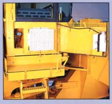
The efficient climate control system with replaceable air filters, gives you the ideal working temperature in all possible conditions. A total of 14 adjustable vents, including a 4-speed fan, circulates dust-free air evenly throughout the cab.
