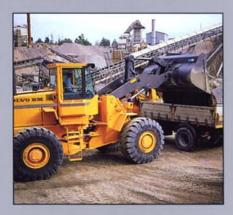
TP-linkage gives both high breakout torque and parallel action within the whole lifting range. High, controlled tilt speeds contribute to short cycle times and a minimum of spill.
