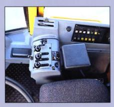
The hydraulics are finger-tip controlled. And there's even a control for forward and reverse\*), kick-down and engine braking/downshifting on the hydraulic console so the operator needn't move his hands.
