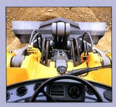
Large windows and the loader units "clean" design allows for good visibility over the loader's bucket and wheels. Positioning of the exhaust pipe and rear wipers gives clear rear window visibility.
