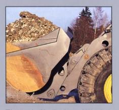
The standard bucket is specially adapted for the carrying position and is held in place against the mechanical stops by substantial hydraulic forces. This provides very good stability and a minimum of spill during load and carry work.
