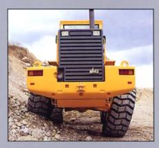
The rear axle can oscillate 15° without shifting the machine's centre of gravity. This rear axle oscillation also means that all the wheels remain in contact with the ground even when operating in uneven terrain.
