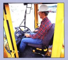
The seat, steering wheel, pedals and controls are ergonomically well-placed. The seat is adjustable to suit the weight of the operator and the wheel can be tilted and moved up or down\*). The Care Cab enables every operator to find the perfect driving position.
