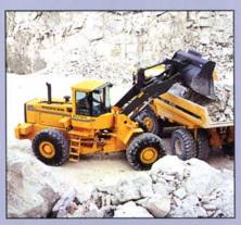
The new loader unit TP-linkage (Torque Parallel) is designed for demanding production work such as quarrying. TP-linkage brings together the best from Volvo BM's parallel-system with advantages from the traditional Z-bar linkage.
