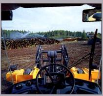
Thanks to the loader's compact design and the large, curved wrap-around front windshield, you enjoy excellent visibil-ity over the wheels and attachments. Large well-placed, rear-view mirrors provide excellent visibility to the rear without blocking the view ahead.
