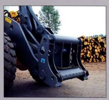
VME's hydraulic attachment bracket is the key to the loader's great versatility. The wide range of attachments together with the hydraulic attachment bracket enable you to switch quickly from one type of job to another.
