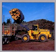
High breakout torque within the whole lifting range enables you to handle heavy timber loads with great precision. You maintain 85% of the breakout torque up to the top position giving you total control of the load throughout the whole lifting range.
