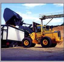
The highly placed loader arms give you a long reach and a high lift capability which facilitates loading high vehicles, such as when you're working with the high-dump bucket. Thanks to the height and angle of the front windshield, you can see the bucket clearly, even in the highest postion.
