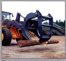
The working hydraulics in the L150 and L180 are pilot-controlled with finger-tip ease. This gives you precision control whether you're carrying a whole cluster of logs or just one. That's a big advantage when cleaning up in the yard.
