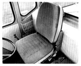
The seat can be moved forward and back, and the backrest angle can be adjusted. The seat spring action is adjustable, with an indicator to show when it is set correctly for the driver's weight.
