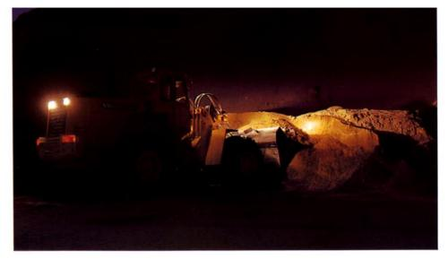
One of the advantages of the new Volvo BM advanced side-arm system is the outstanding forward visibility it gives over the work area. And the matt black of the arms permits the use of powerful halogen lamps as floodlights without the problem of glare.
