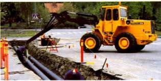
Good lifting height and long reach make the loading of wide vehicles easy. In addition, the 4300 B has a good parallel side-arm action, for safe handling.
