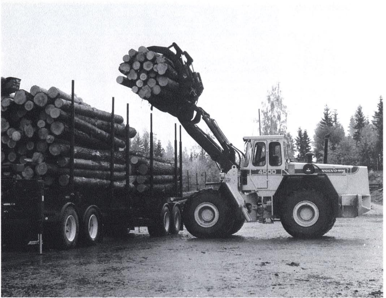
Long reach and good lifting height are an asset for loading or unloading timber vehicles. These features enable the work to be carried out quickly and surely. The excellent breakout forces, even in the top position, permit superb handling of roundwood.
