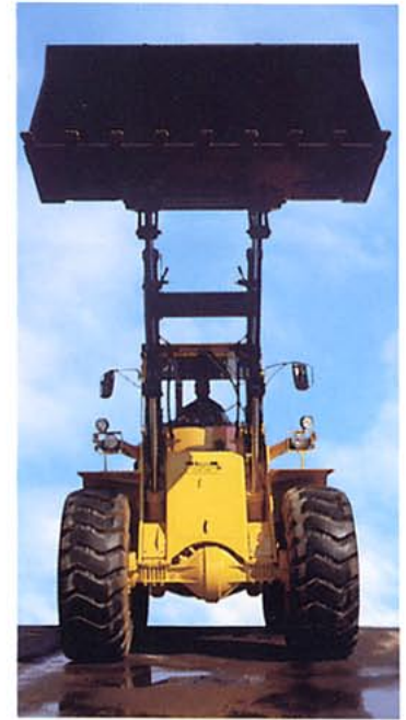
The symmetrical attachment of the cylinders gives very good reliability and extra good visibility through the loading unit.
