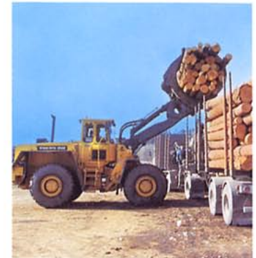
High tilt and rollback forces throughout the lift-arm movement permit effective, controlled unloading of timber trucks.
