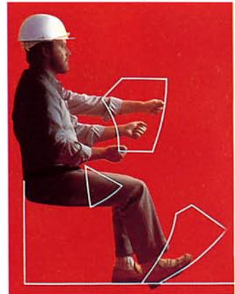
The cab is ergonomically designed to enable the operator to achieve high performance with low fatigue. Controls and instruments are ideally located.
