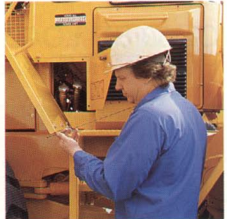
All oil checks can easily be performed from ground level.
