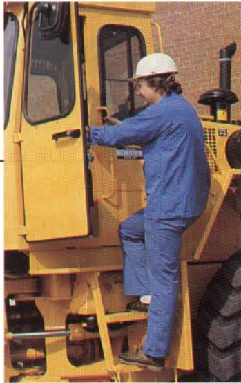
Conveniently located grab bars and footsteps make it easy to enter and leave the cab.
