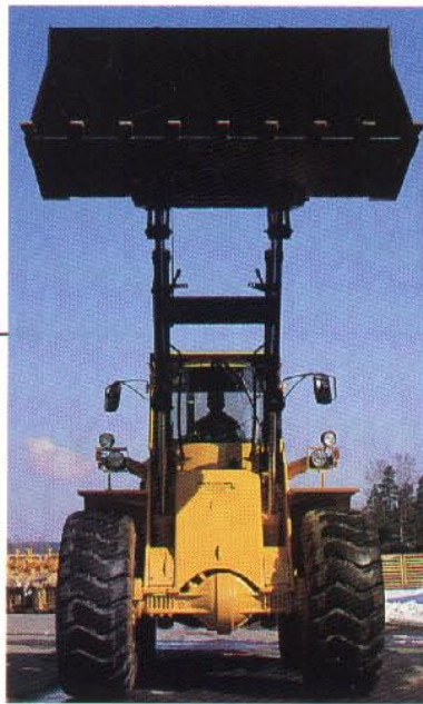
The symmetrical attachment of the hydraulic cylinders provides good reliability and extra good visibility through the loader unit.
