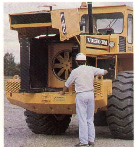
Large access panels and platforms permit easy and safe inspections.
