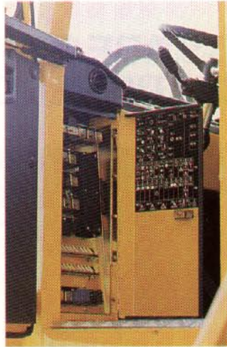
The electrical distribution box is logically arranged and conveniently located inside the cab.
