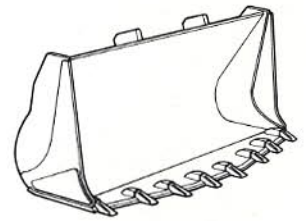
Truncated V-lip with teeth. Suitable for hard and stony material, hard gravel and blasted rock.
