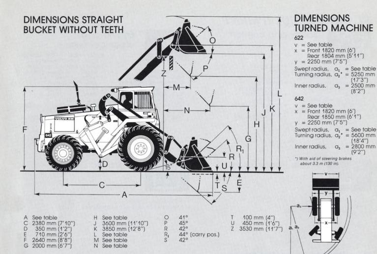
The specifications pertain to a standard machine equipped with a 1.0  $m^2$  (1.3  $yd^3$ ) straight bucket without teeth and tyres 16.9—30/14 front and 12.5—20/10 rear for the 622 and 12.4—24/12 for the 642.
