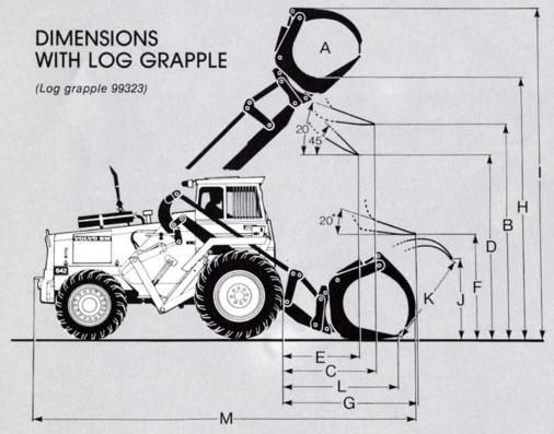
A = 0.8 m² (8.6 sq ft) B = 3500 mm (11'5") C = 1340 mm (4'5") D = 3070 mm (10'1") E = 1100 mm (3'7") F = 1540 mm (5'1") G = 2130 mm (7') H = 4000 mm (13'1") I = 5300 mm (17'4") J = 2000 mm (6'7") K = 2030 mm (6'8") L = 1620 mm (5'4") M = 6075 mm (19'11")
