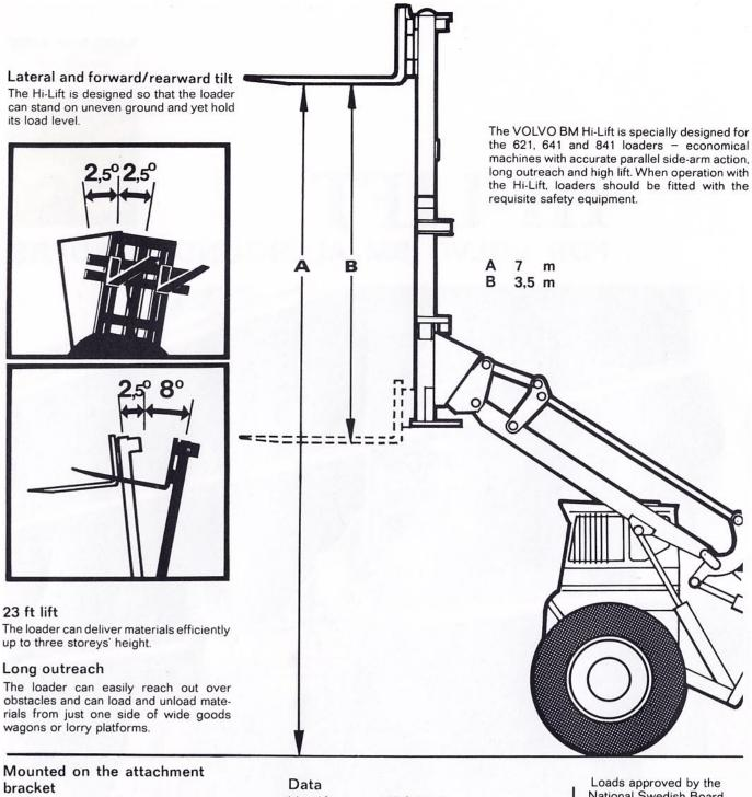
The Hi-Lift is mounted on the attachment bracket of the loader, and rapid switches can therefore be made to other "Allrounder" attachments for other jobs.
