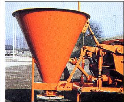
Three-point hydraulic attachment: sand, salt or fertilizer spreader.
