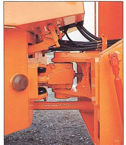
Built for extreme resistance – a low-maintenance forged articulating – oscillating joint.
