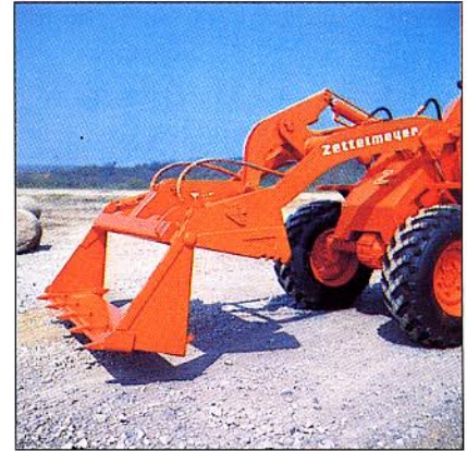
The clam bucket does 4 jobs in one: excavating, loading, grabbing and levelling.
