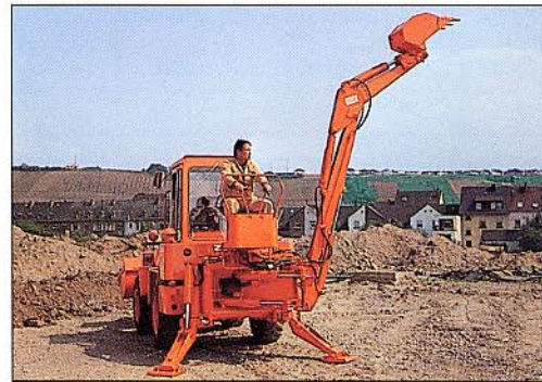
Side shift adjustment is continuous up to 1.10 m operated from the driver's seat for excavator attachment.
