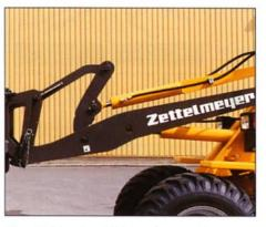
Parallel loader-linkage for good loading fork features - parallel lift of the working equipment for smooth loading and unloading at every lift height.
