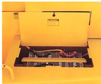
Battery box positioned for convenient inspection.
