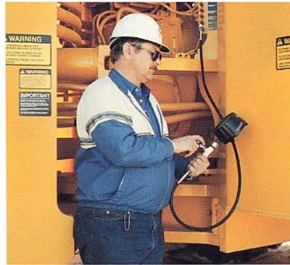
Quick-connect, remote pressure check ports save time and labor.
