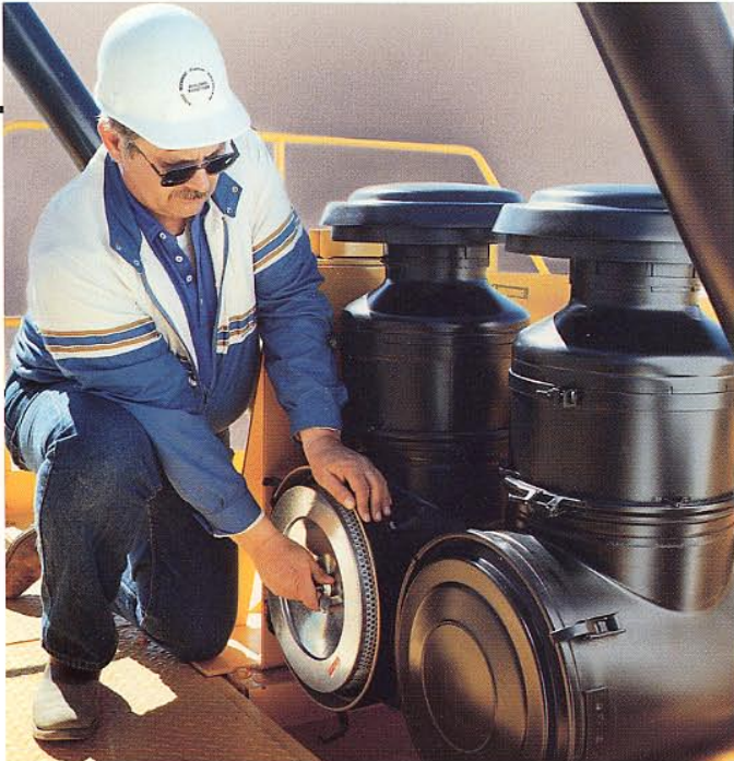
Air cleaner restriction sight gauge / service platform.
