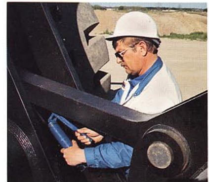
Grease fittings grouped so they can be lubed from four ground level locations.
