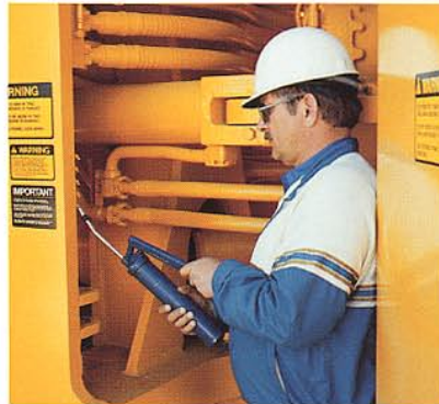
Center hinge lube manifold.
