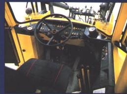
With the controls at his fingertips, the operator can now change hydraulic powered attachments without leaving the cab.
