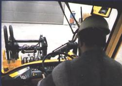
A simple touch of a dash mounted rocker switch while moving the 3rd valve lever activates the mechanism which connects the male and female hydraulic couplings.
