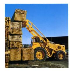
The LM 840 is well suited to the stacking of palletized goods and sawn timber, thanks to the combination of good reach and generous lifting height. The machine can stretch high over the growing stack, which provides a support when placing the final pallet or package.
