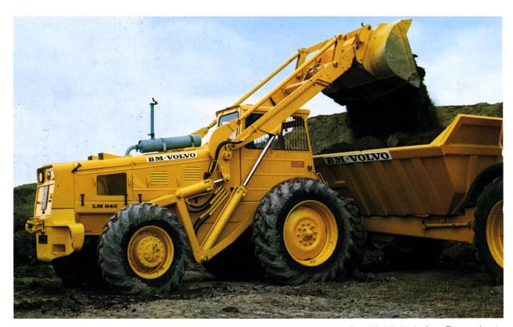
The LM 840 loads fast. This is due to excellent bucket filling, quick maneuvering assisted by the tight turning radius, and simplified load distribution as a result of long reach.
