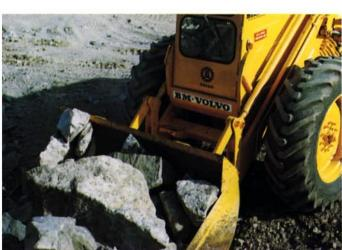
The remarkably high penetration force of the LM 840 assists effective bucket filling. In combination with the large wheels and ideal weight distribution (= low ground pressure) and balanced transmission (= stepless torque multiplication, plus differential-lock feature) the result is a high-output machine that maintains performance even under adverse conditions.
