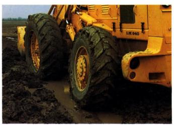
On loose or slippery surfaces the specific ground pressure and contact area are vital factors in the machine's ability to keep moving. The LM 840 fully satisfies these conditions and, despite its weight, can carry on in places where many machines would experience difficulty in working.
