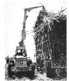
Outreach at lift height of 6 ft 6 in (2 m): Bucket capacities 4 ft 7 in (1.4 m) 1 1/4—4 yd³ (0.95—3.0 m³) Indicated data for rear tires without calcium
