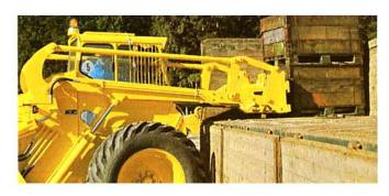
An LM 640 has no trouble lifting loads over wide platforms and onto high stacks, thanks to the geometry of the lifting gear. This affords generous reach and high lift, with good visibility at all positions. In off-the-road work
