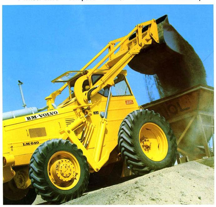
The BM-VOLVO LM 640 is an easily manoeuvred, 4-wheel drive loader featuring torque converter and hydraulically operated gearbox. The large wheels and traction power of the machine eliminate the risk of bogging-down when ground conditions are bad. This loader therefore stands out in its class as a tool for earth-moving jobs, loading and general-service work.
