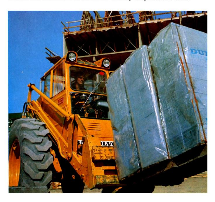
High lift, long outreach, easy handling and a tight turning circle make the LM 620 a truly versatile loader. The comfortable, crash-proof driver's cab and hydraulically operated gearbox without clutch pedal ensure a high degree of convenience and safety, improved performance and less strain on the driver.
