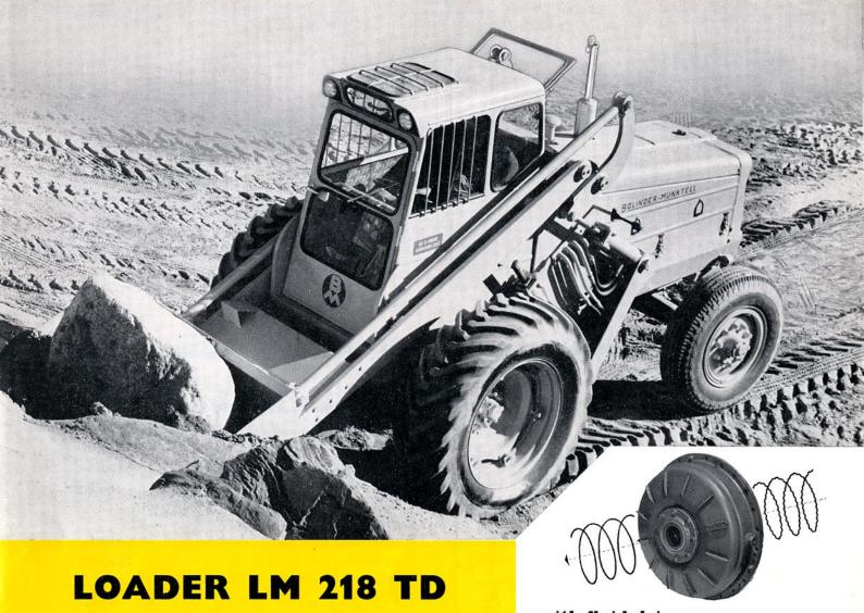
Bolinder-Munktell's loader is fitted with a rugged 13" dry-plate clutch as standard. This clutch can be used in conjunction with a fluid drive unit for *smooth starting* when heavily loaded — and to permit starting without wheelspin. This is made possible by the cushioning effect of the fluid drive, which varies in proportion to engine revolutions. At 600 r. p. m. the loader is stationary — at 1800 r. p. m. more than 98  $^{0}/_{0}$  of the engine power is transmitted to the driving wheels.
