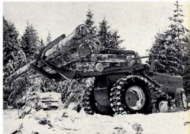
Skidding and loading logs and pulpwood, equipped with half-tracks and log or pulpwood fork.
