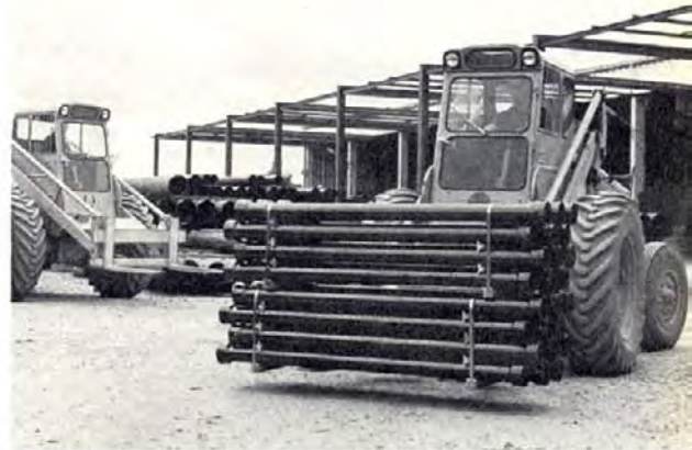
Handling bundled and palletted freight, sawn timber, barrels or drums, with regular angle-tine and drum forks.
