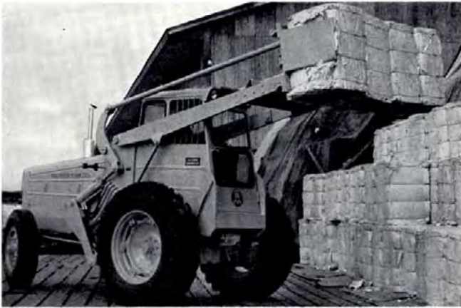
Handling baled goods with the hydraulically operated clamp.
