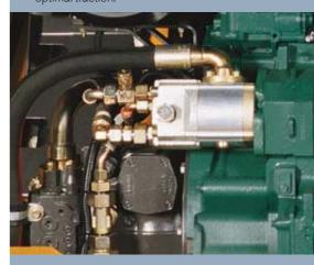
Separate hydraulic pumps provide fast cycle times.
