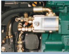
Separate hydraulic pumps provide fast cycle times.
