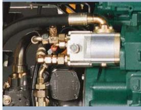
Separate hydraulic pumps provide fast cycle times.
