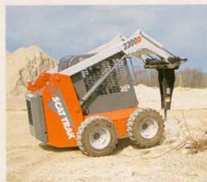
The 22 GPM hydraulic pump delivers plenty of power for optional attachments.
