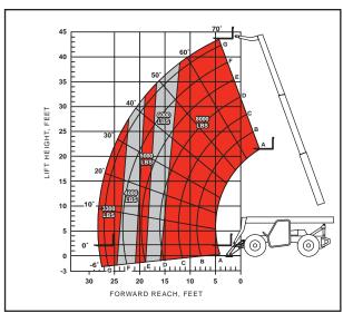
Always read and understand the published rated load capacity for the material handler model you are operating and do not exceed it. Load ratings per ASME B56.6 — 1992.
