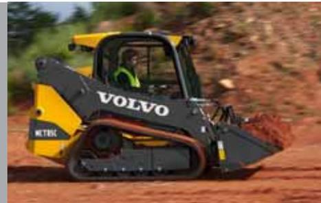
Volvo assisted attachment bracket allows the operator to change attachment from the seat
