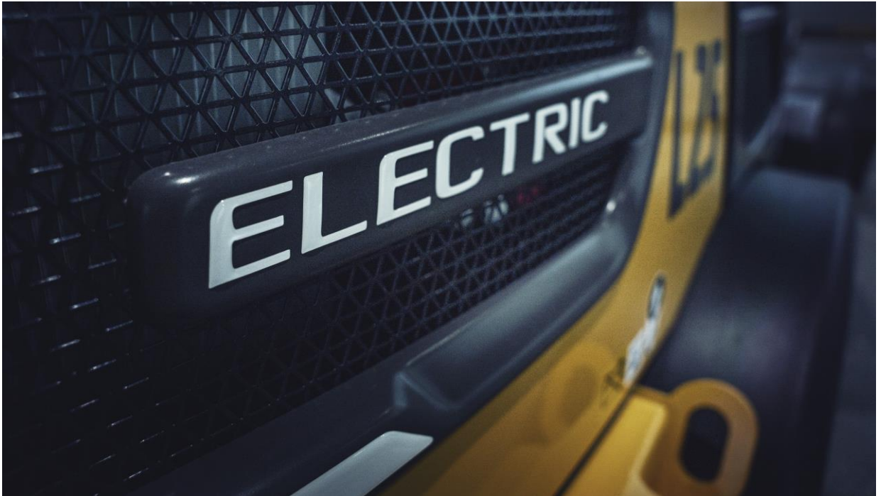
The Volvo L25 Electric packs a battery capacity of 39kWh so it can work continuously for six hours before it requires charging
