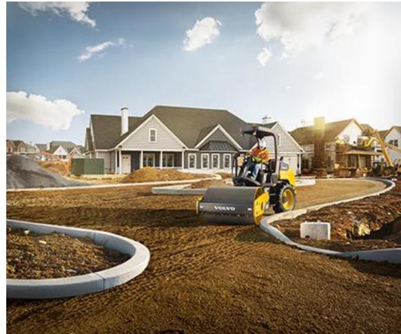
The Tier 4 Final compliant SD45B, meanwhile, is a single drum compactor that is designed for commercial and residential site development, utility installations, driveways and landscaping jobs. Providing up to 12 degrees of oscillation and 41 degrees of frame articulation in each direction, the SD45B offers the stability and versatility required to compact in confined areas.
