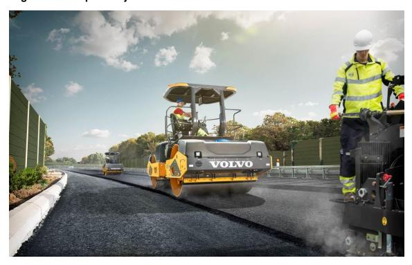
From highways to airport runways, the Volvo DD120C and DD140C are designed to achieve a smooth, even mat finish in fewer passes — all without compromising fuel-efficiency. With operating weights of 27,700 pounds and 30,486 pounds, combined with rolling widths of 79 inches and 84 inches, respectively, the DD120C and DD140C compactors deliver the performance needed for large jobs.
