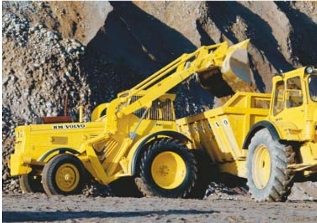
engine. The Volvo motor was rated at 110 horsepower. The LM 642 was the last Volvo wheel loader to use rear wheel steering and it remained in production until 1983.
