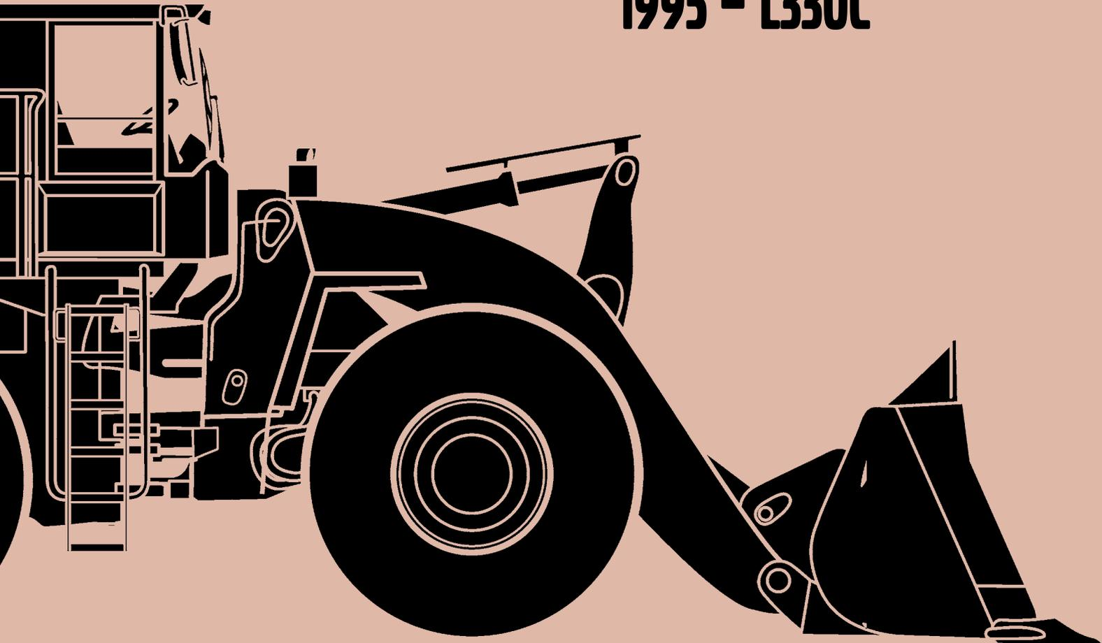
● Operating weight: 46,9–51,4 t (103,320–113,320 lb)    ● Bucket size: 6,1–12,7 m<sup>3</sup> (8.0–16.6 yd<sup>3</sup>)    ● Engine, rated output: 366 kW (498 hp)
