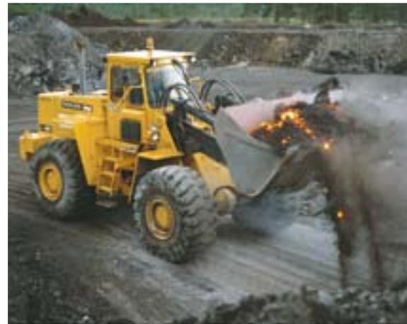
eliminate rocking, both of which occur when operating on uneven ground. The Boom Suspension System gives faster cycle times, less spillage and improved operator comfort.
