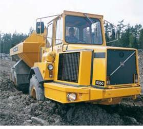
And development of the 5350 continued: a B-version was introduced in 1982, with new axles and disc brakes on all wheels. The following year saw the launch of the 5350 with six-wheel drive, and 1984 saw introduction of a machine adapted for mines and tunnel construction.
