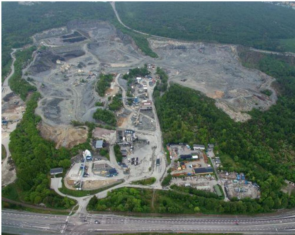
Vikan Kross is Skanska's second largest quarry. It is located in Gothenberg, Sweden. It has been in operation since the early 1960s and plays a major role in the development of the area. The Vikan Kross quarry produces stone materials in various dimensions for building and road construction projects. It also sells materials to asphalt and concrete plants.
